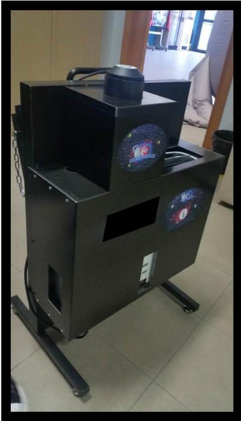
Particular system of our production of computerized digital video projectors, created for the projection and reproduction of effects and animations of large field ( $170^\circ$ ) inside of the planetarium or hemispheric domes of any kind.
